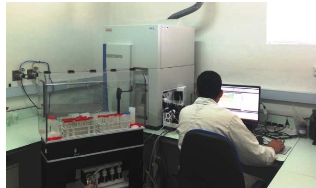
ICP-MS with auto-sampler for metal analysis in water.
