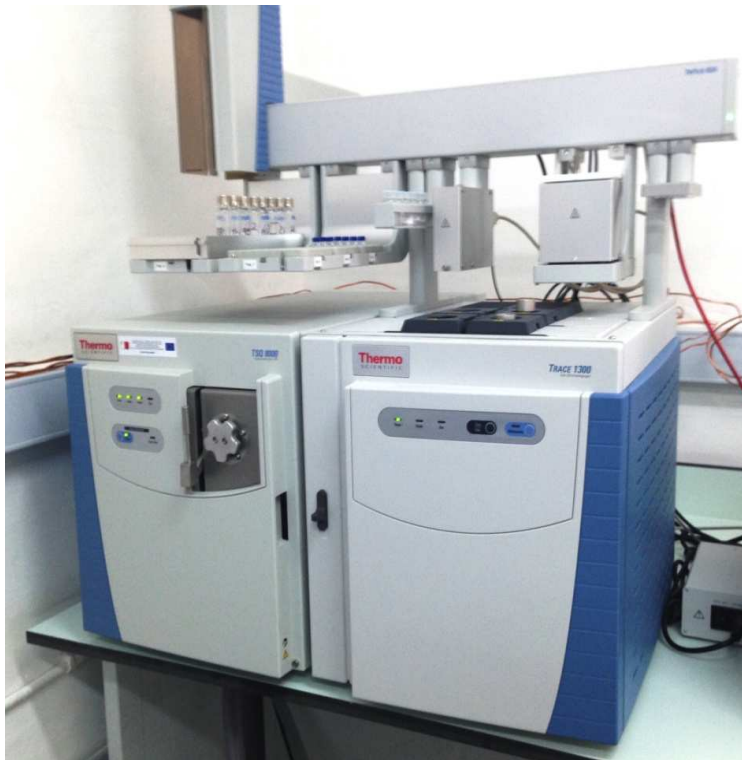
GC-MS/MS with auto-sampler for organic analysis in water.
